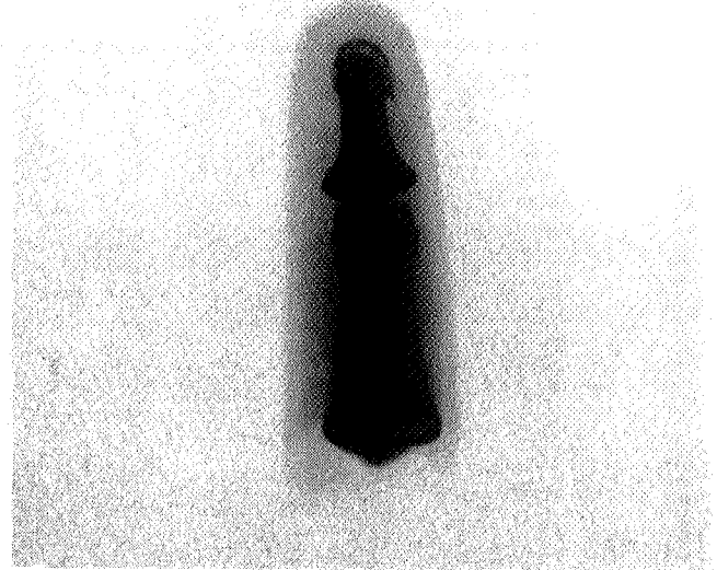
Figure 8. Image of an Alderson Phantom Finger using the Radiographic Inspection System (Faxitron)
