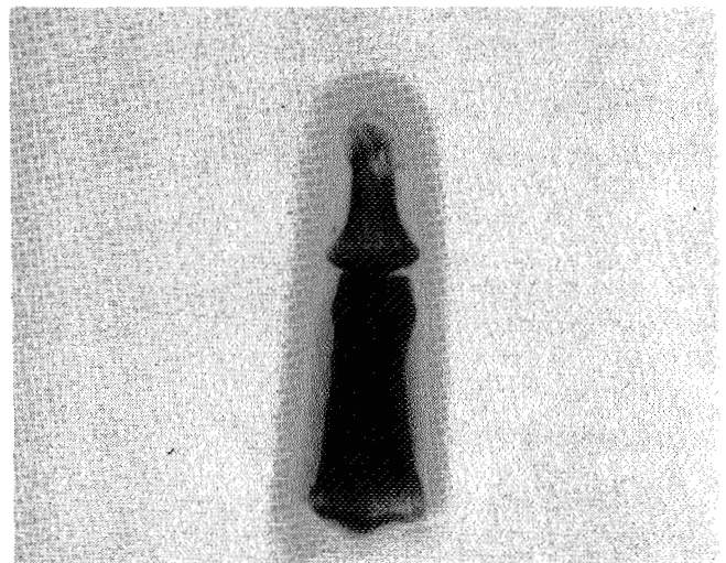
Figure 5. Image of an Alderson Phantom Finger using a Medical Radiographic Unit
