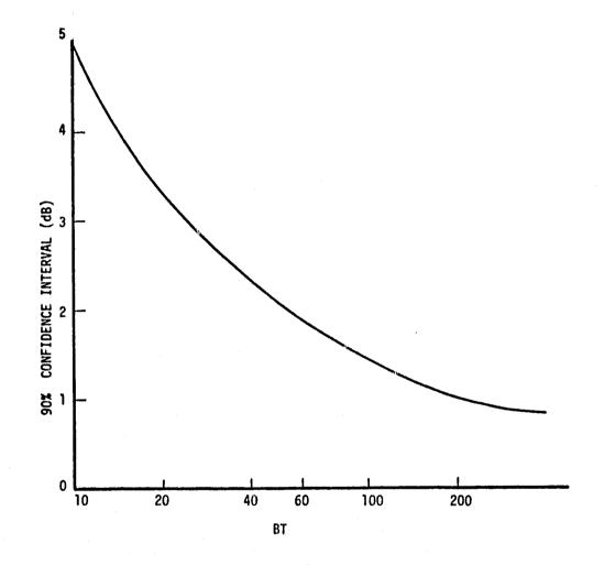
FIGURE 3.4 THE IMPROVEMENT IN PRECISION WITH THE TIME BANDWIDTH PRODUCT
