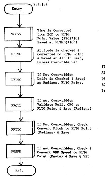
FLTME: ;Gell Time ALT: ;Altitude DRFT: ;Drift (RAD) ROLL: ;Roll (RAD) PITCH: ;Pitch (RAD) VEL: ;GND Speed · 1
