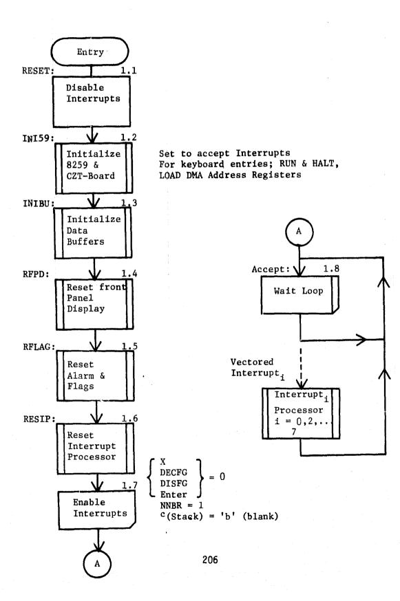
RESET MODULE, C- and L-Band Scatterometer Data Processor
