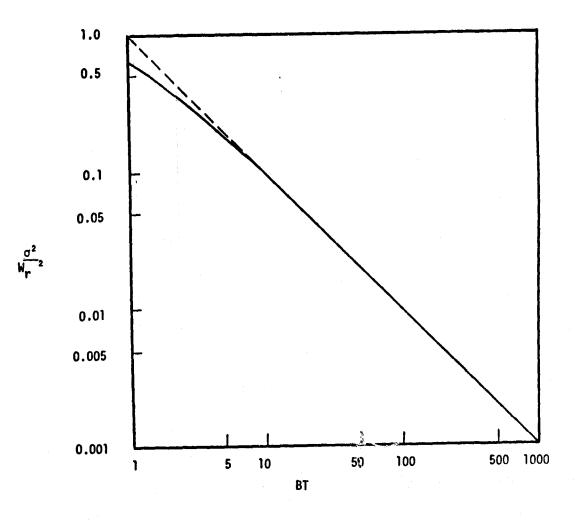
FIGURE 3.3 THE VARIANCE RATIO AS A FUNCTION OF INTEGRATION TIME-BANDWIDTH PRODUCT (FROM REFERENCE [2])
