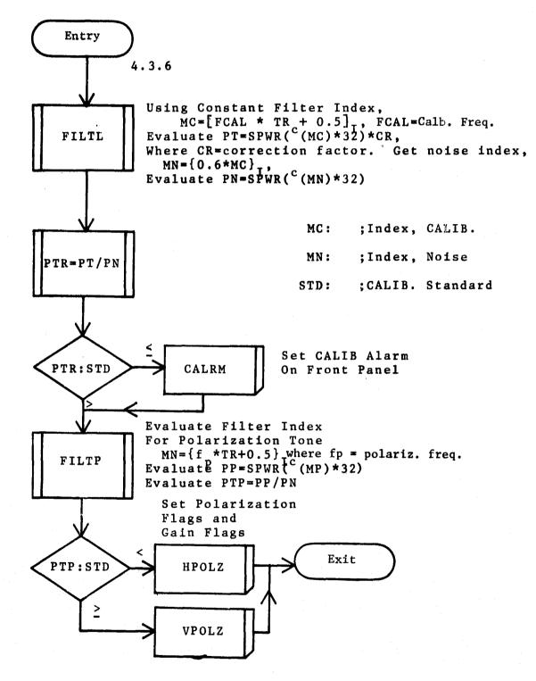
INTERRUPT-1 PROCESSOR, RUN Module, SIGM2 Module POWER; Computer Spectral Power for Each Doppler Band
