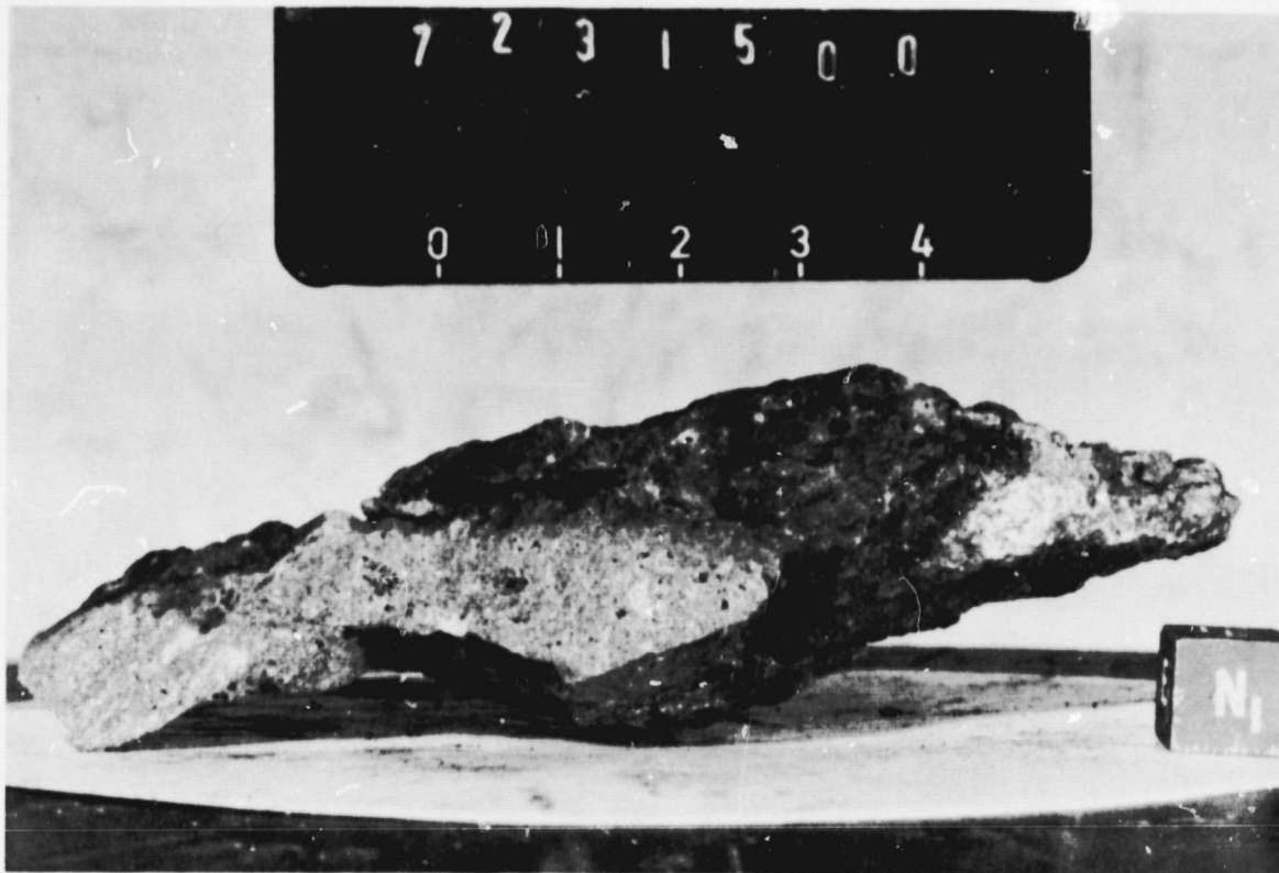
72315- A clast-bearing impact-melt breccia which is compositionally similar to rocks from both the North and South Massif at Apollo 17 but which displays a slightly different texture from other rocks in the suite. The rocks may have been produced by the Serenitatis impact.
