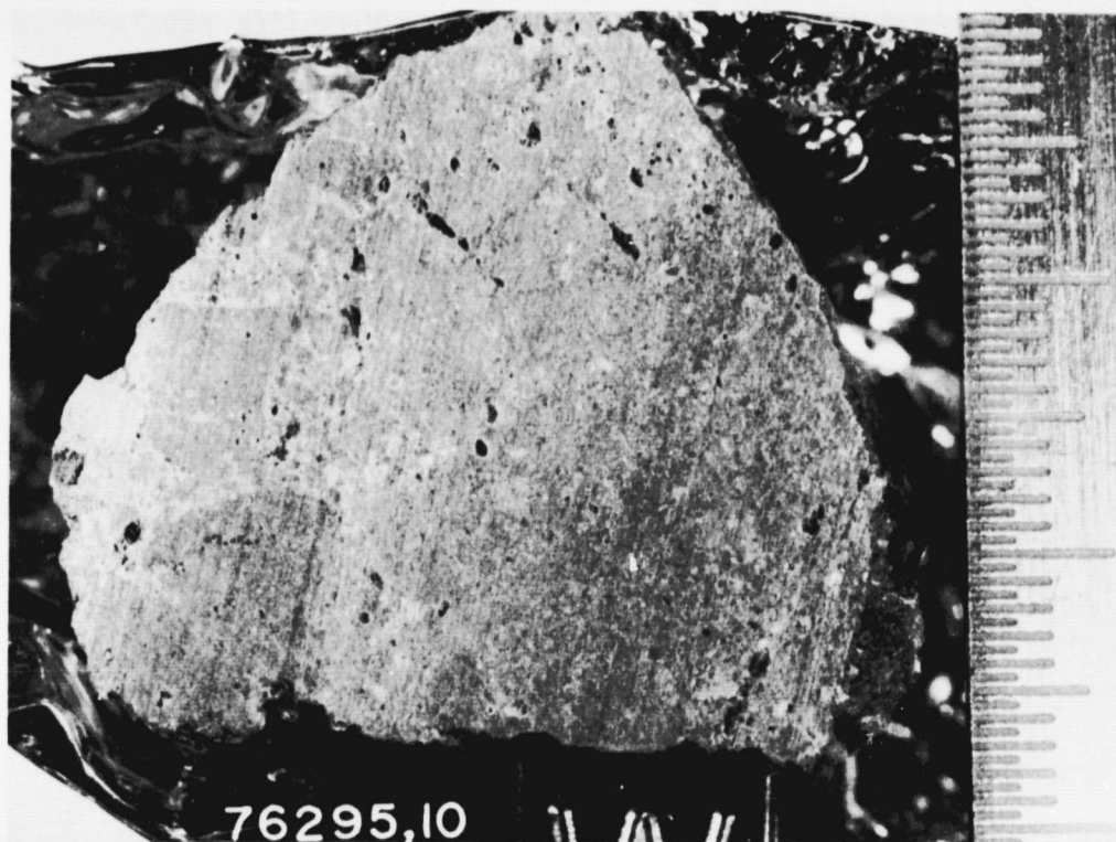
Sample 76295 is a light to medium bluish-grey, wedge-shaped rock (10x6x3.5 cm) which was chipped from the boulder farthest upslope in a group of five boulders at Station 6.
