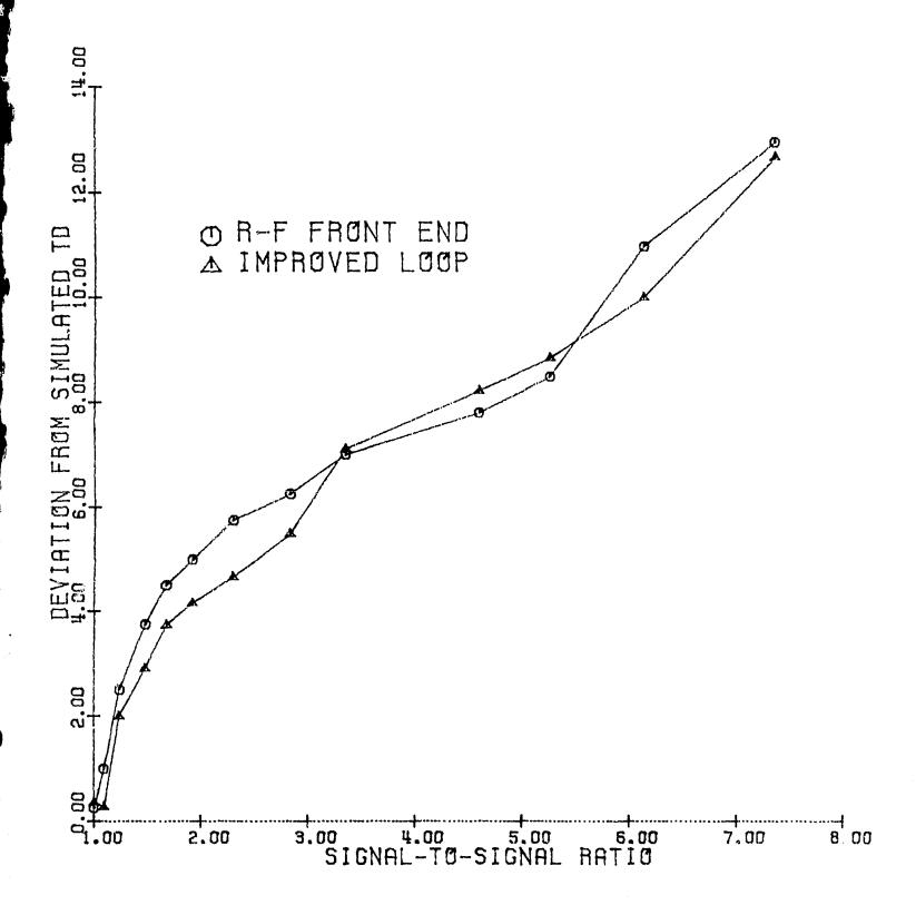
Figure 5. DPLL and RF Front-End Characteristic Curves Vs. S/N.
