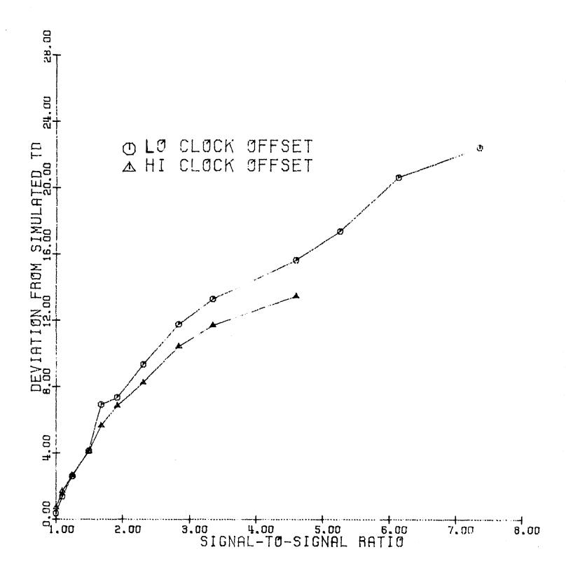
Figure 4. DPLL Characteristic Curves with Different Clock Offsets Vs. S/S.
