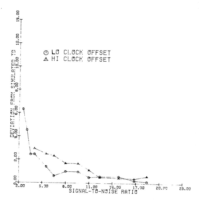
Figure 3. DPLL Characteristic Curves with Different Clock Offsets Vs. S/N.
