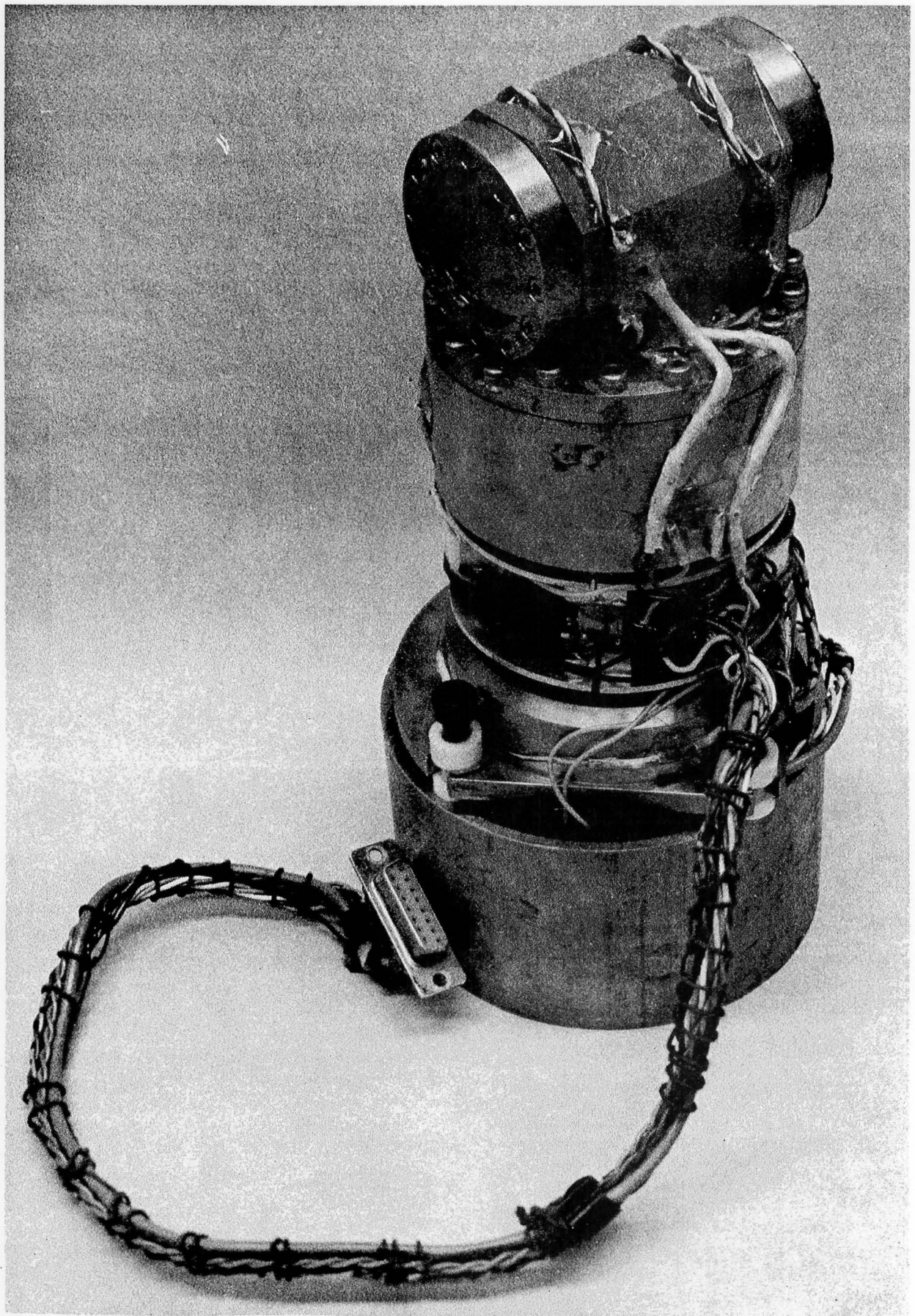
Figure 3-1. Nimbus "F" Pressure Modulator Cell and Optical Head
