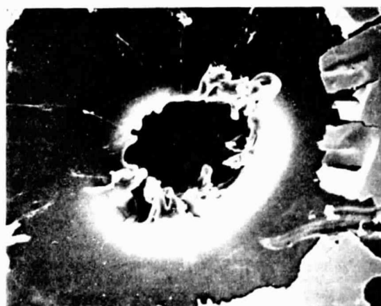
d. Scanning electron micrograph of damage to silver side. (225 X)
