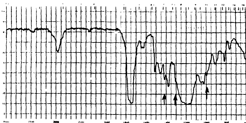
Figure 32. Infrared spectra of the phenol-formaldehyde resole through cure.
