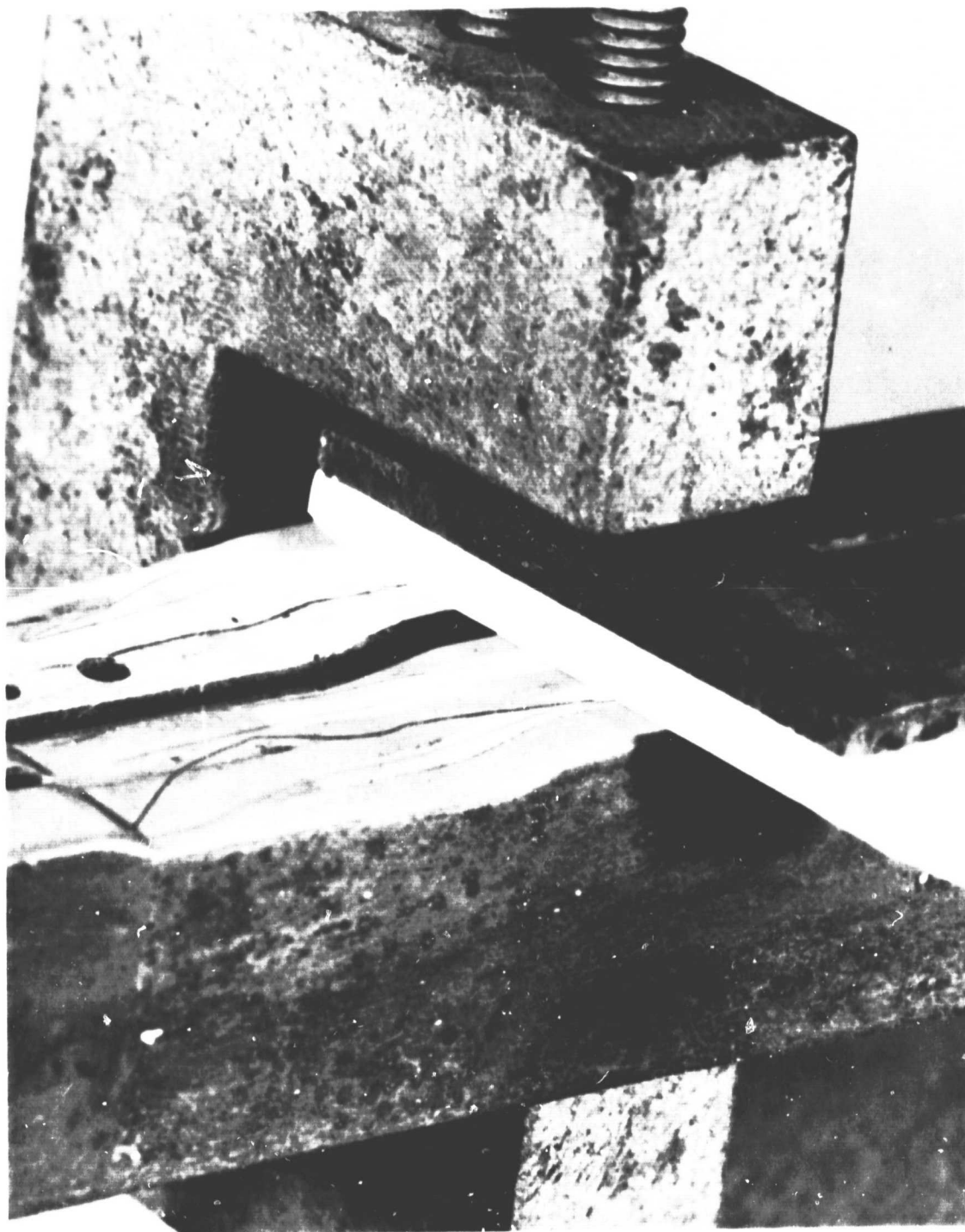
Figure 5 Lead Wires (0.075 mm diameter) - The lead wires are shown clamped to the thin films on the simulated blade in preparation for diffusion bonding.
