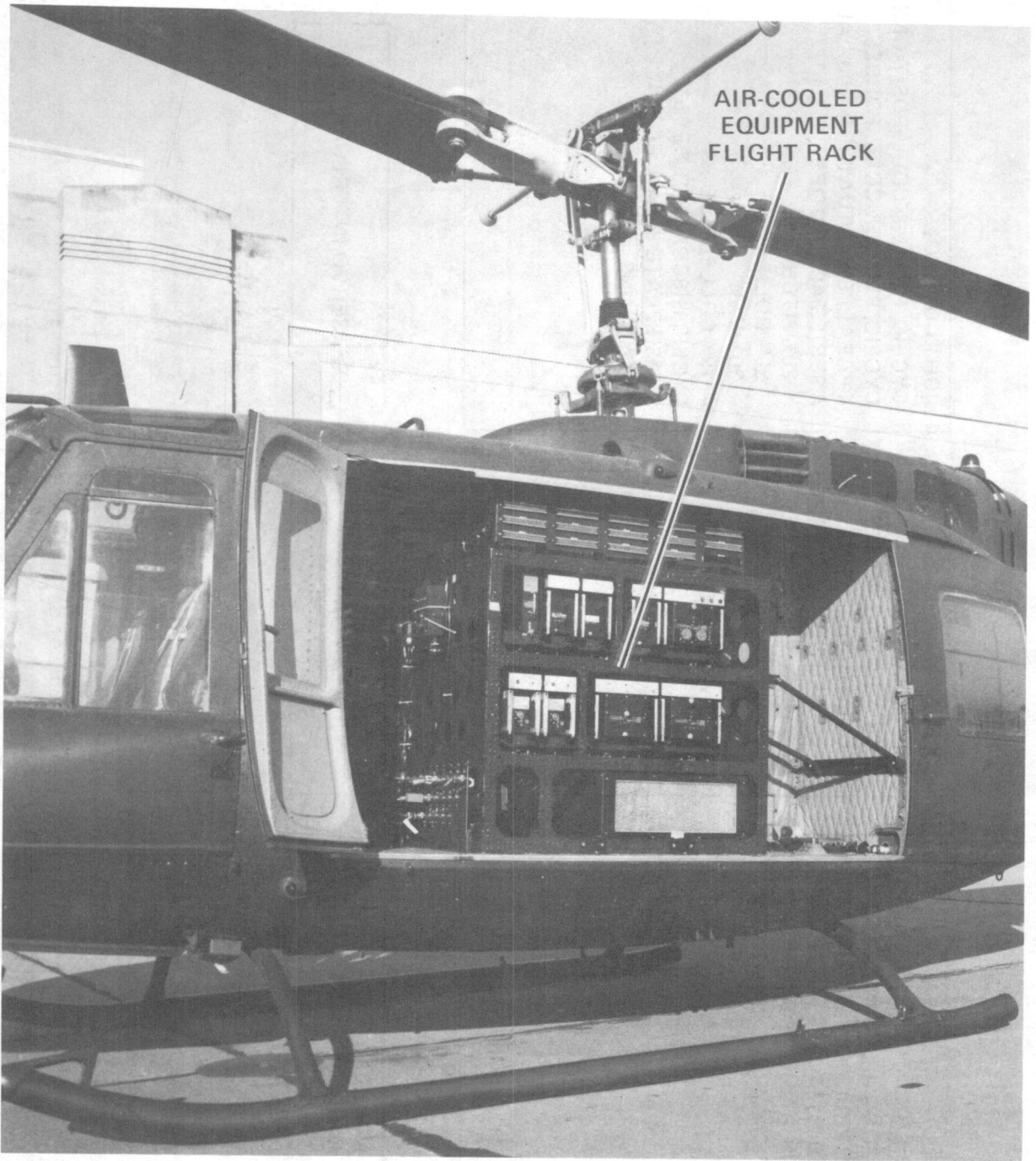
Figure 2.— Installation of the air-cooled equipment flight rack.
