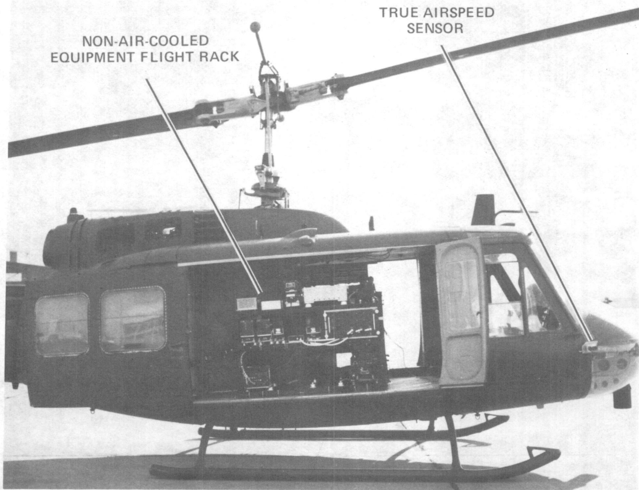
Figure 3.— Installation of the non-air-cooled equipment flight rack.
