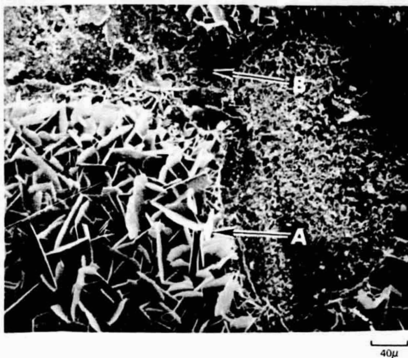
a. A. Chromia crystals produced by molten salt effects B. Matrix scale
