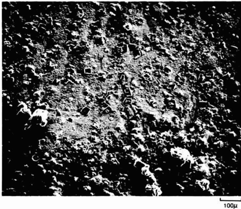
FIG. 23 B-1900 oxidized at 700°C.
