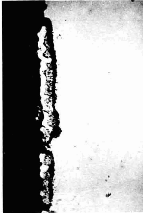
D. Internal oxidation.
