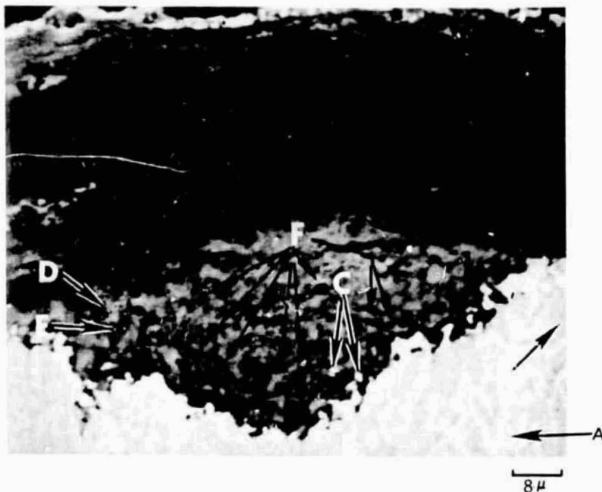
FIG. 41 Pitting Attack of CoCrAlY
