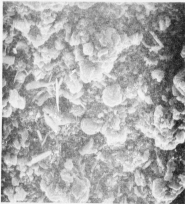
(b) AFTER 984 hours AT 650° C, 3000X, 30° TILT.
