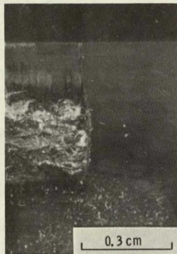
(a) FATIGUE SPALL.
