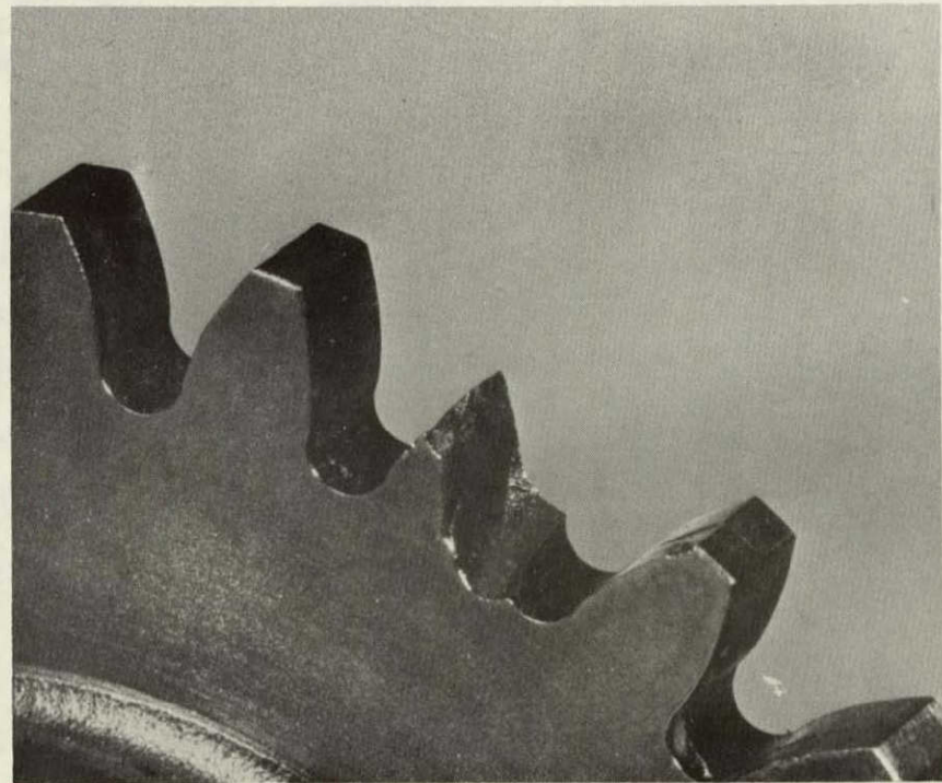
Figure 12. - Gear tooth fracture through a fatigue spall of NASA heat treated modified Vasco X-2, maximum Hertz stress, 1.71 \times 10^9 N/m 2 (248 000 psi) speed, 10 000 rpm.
