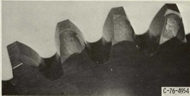
Figure 9. - Typical fracture of modified Vasco X-2 gear teeth with NASA specified heat treatment carburized on all sides.
