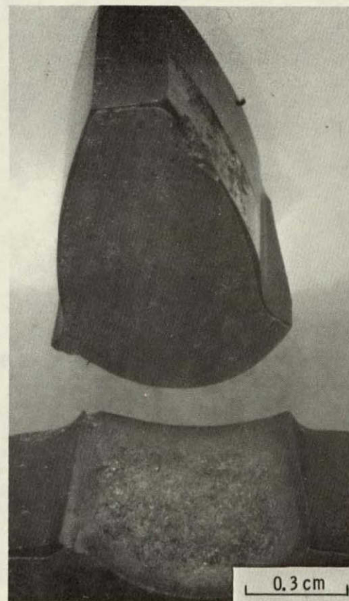
Figure 8. - Typical tooth bending fracture on CBS 600 after running with a fatigue spall; speed, 10 000 rpm; lubricant, synthetic paraffinic oil with additive package.
