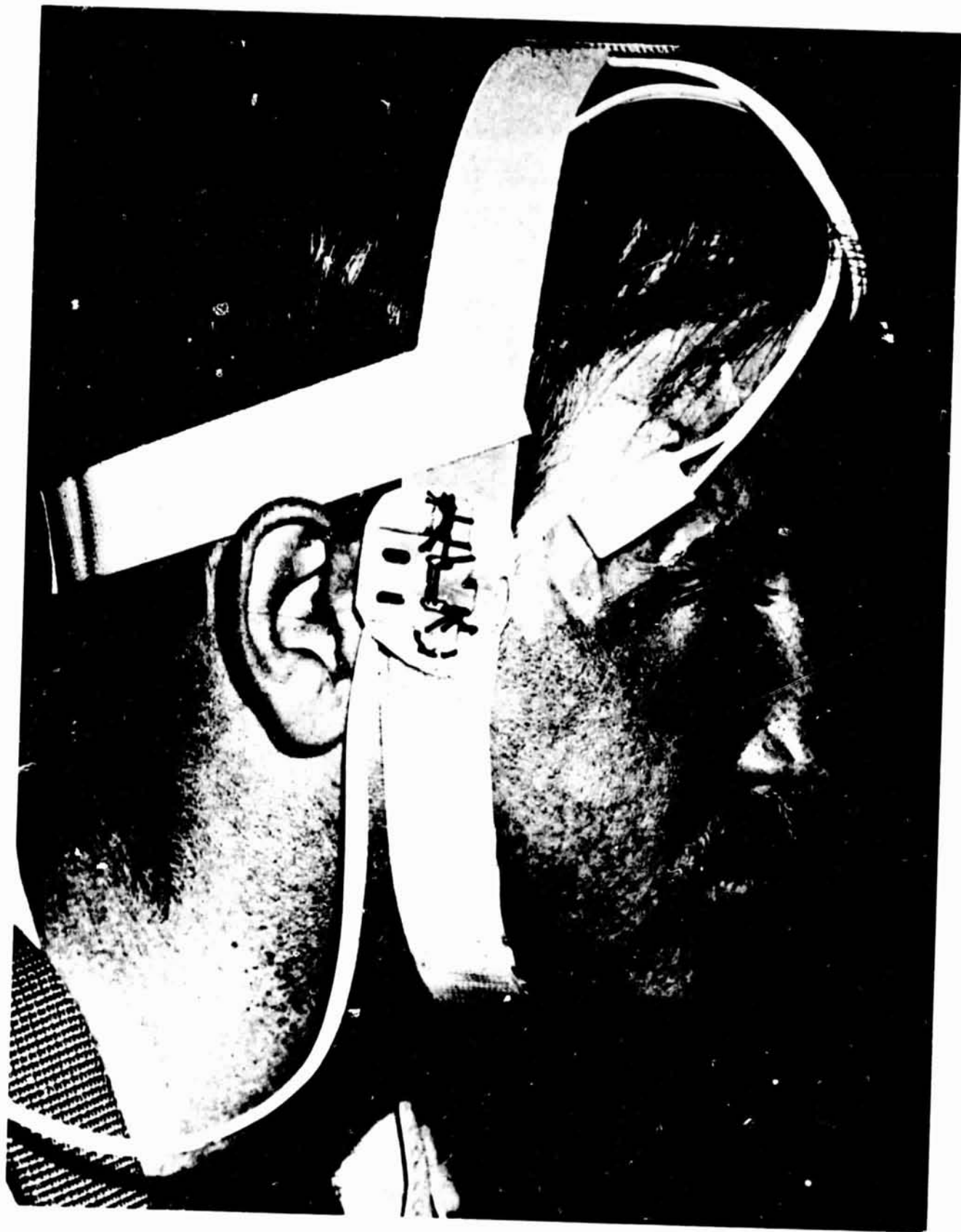
Figure 19. Velcro harness for eye level arterial pressure cell.
