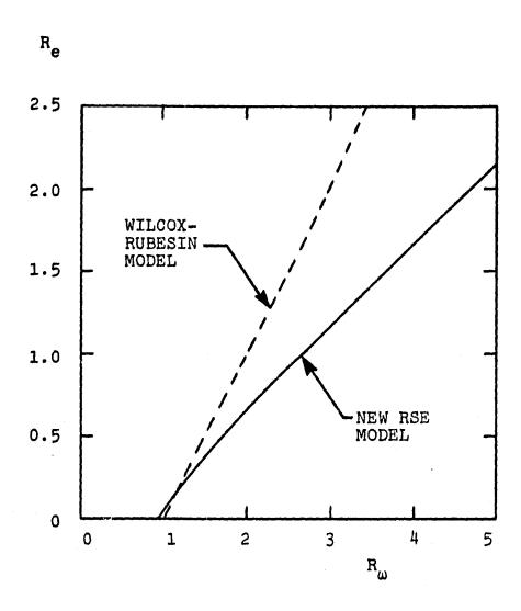
Figure 1. Loci of values of  $\rm R_e$  and  $\rm R_w$  which yield a smoothwall constant in the law of the wall of 5.5.
