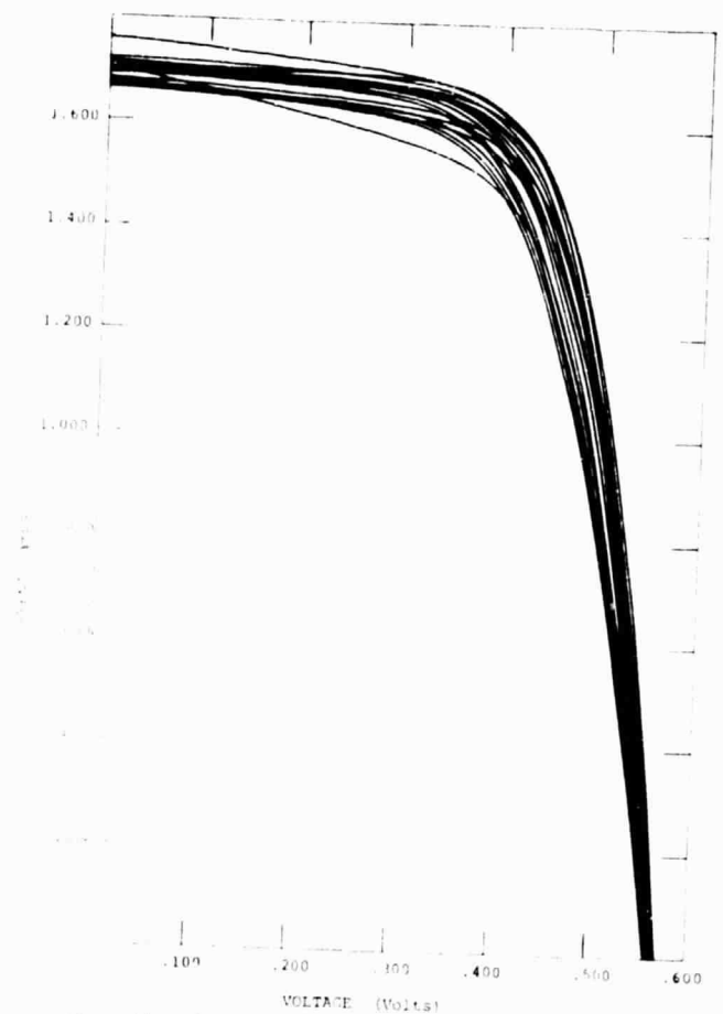
Figure 6: Electrical performance curves for 3.35 inch diameter intermediate gettered (POCl 3 , 875°C) solar cells, Batch P-4.
