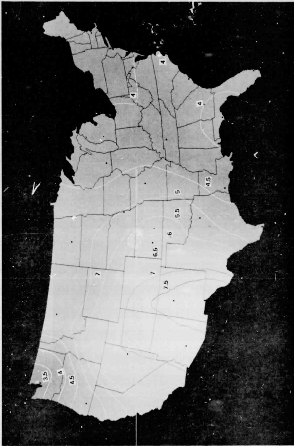
Figure A-16. Data Based on Aerospace Corp. Estimates of Direct Normal Insolation. The Degree of Smoothing of the Surface Increases in Going from Figure A-15 to Figure A-17. Figure A-16 Corresponds Approximately to an Average Nyquist Sampling (See Text).
