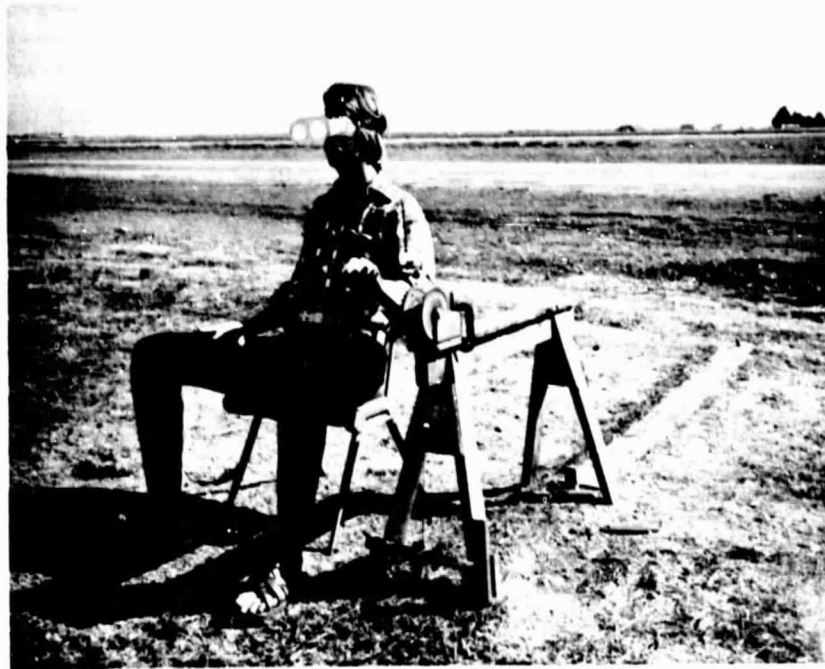
Figure 3.— A person in position to make an angular size judgment. His hand rests on the crank used to adjust the height of the variable triangle. He is wearing the 22.5^\circ FOV goggles.
