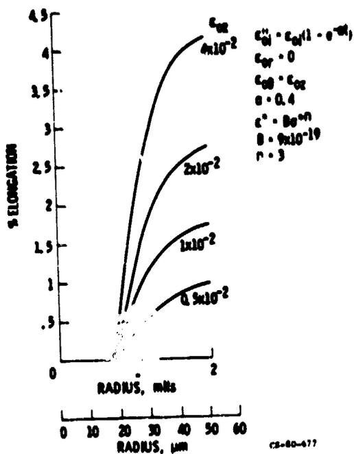
Figure 7. - Calculated percent elongation versus filament radius,  $r$ , as a function of  $E_{0\theta}$  and  $E_{0z}$  (Eq. (1)).
