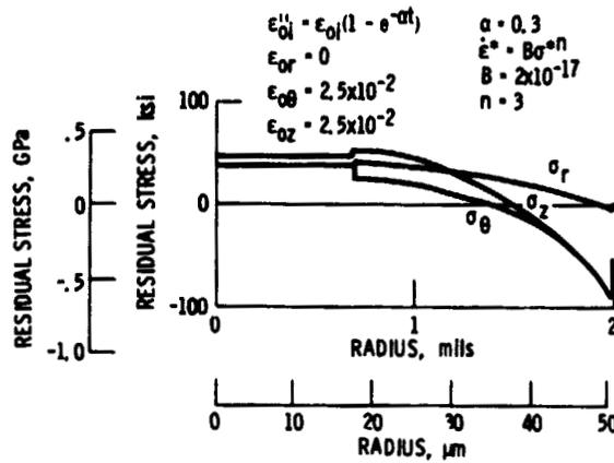
Figure 9. - Calculated residual stresses,  $\sigma_r$ ,  $\sigma_\theta$ , and  $\sigma_z$  versus radial location,  $r$ . The deposition and creep parameters are the same as that for the calculated curve in Figure 8.
