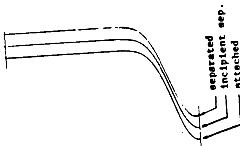
Fig. 6a Streamwise velocity profiles in separation region
