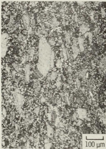
(b) HIP AND FORGED LC ASTROLOY.
