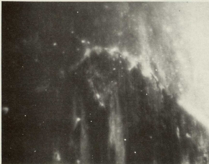
(a) AN SEM MICROGRAPH OF A BALL AFTER HITTING A 6061 ALUMINUM TARGET AT 180 m/sec.
