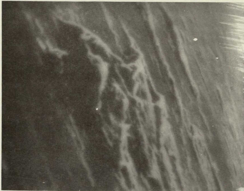
(a) AN SEM MICROGRAPH OF A CHUNK OF TRANSFERRED TARGET MATERIAL AFTER HITTING A 6061 ALUMINUM TARGET AT 180 m/sec.
