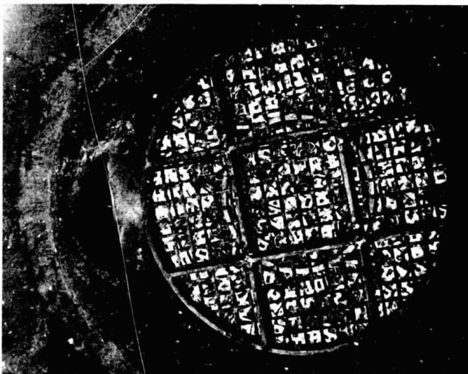
Figure 13-19. Posttest Compacted Bed of Aluminum Ballast Rings
