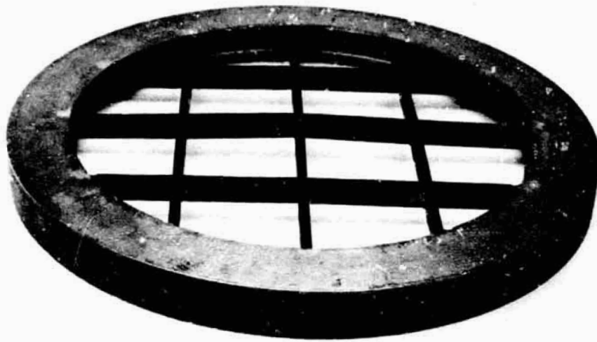
Figure 13-12. Spiral-Wound, Crimped Ribbon Arrester Mounting Ring, Posttest Downstream Side Showing Deformation of Retainer Grid
