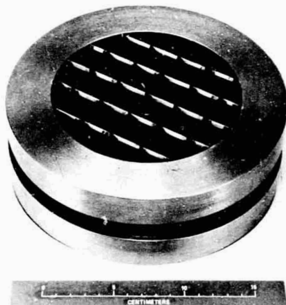
Figure 3-4. Spiral-Wound, Crimped Stainless-Steel, Ribbon Air Flow Straightener
