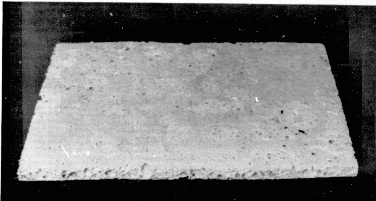
Figure 71. Wall Panel Core by Microwave Process Having Density Less Than 80 kg/m 3 (5 lbs/ft 3 )
