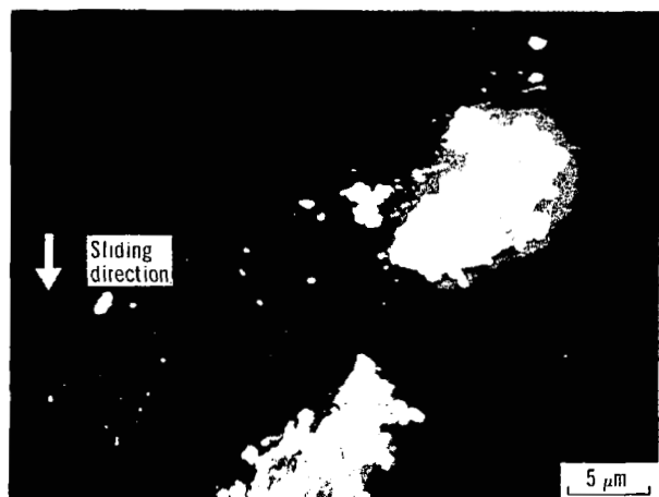
Figure 8. - Wear track on SiC flat showing wear debris and transfer film of 1.02 at.% Ti-Fe pin. Scanning electron micrographs; SiC {0001} surface; number of passes, 10; load, 0.2 N.
