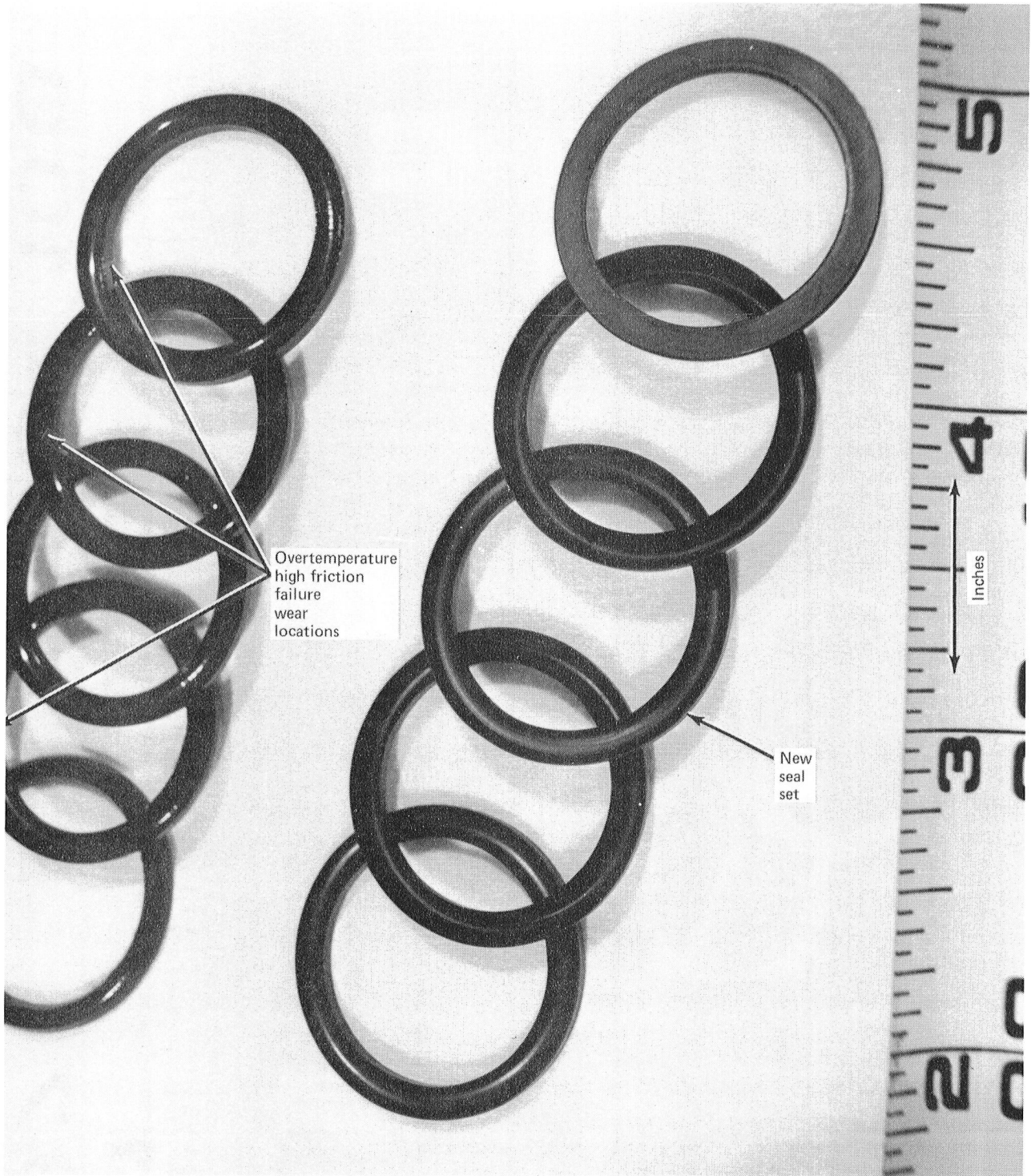
Figure 17. – NASA Chevron Seal Failure
