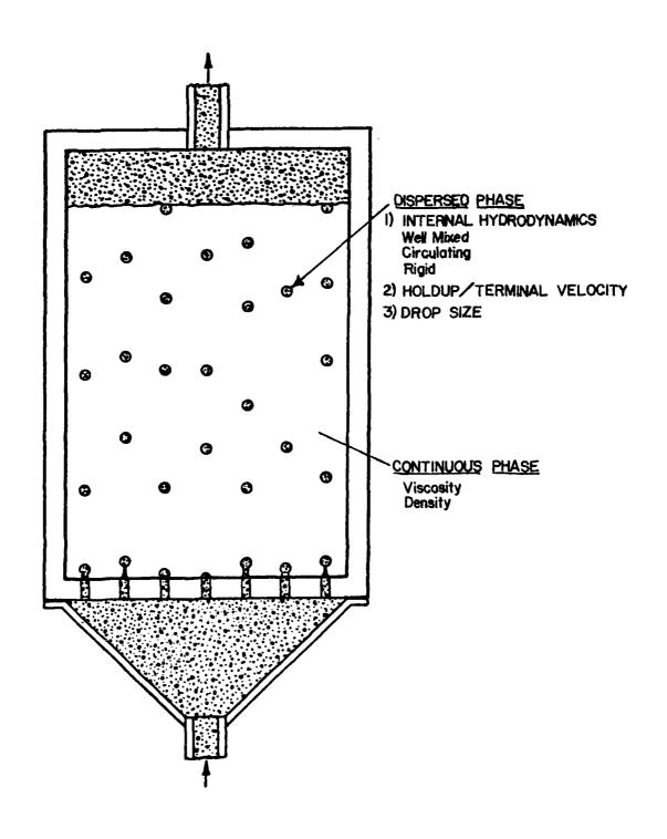
FIG. I MECHANISMS CONTROLLING HEAT TRANSFER
