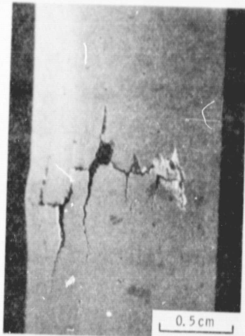
(a) FAILED REGION ON BURNER RIG BAR.
