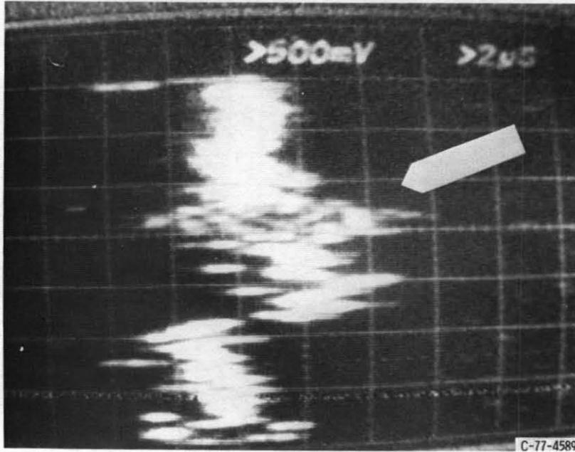
Figure 13. - Initial response of localized choke flutter.
