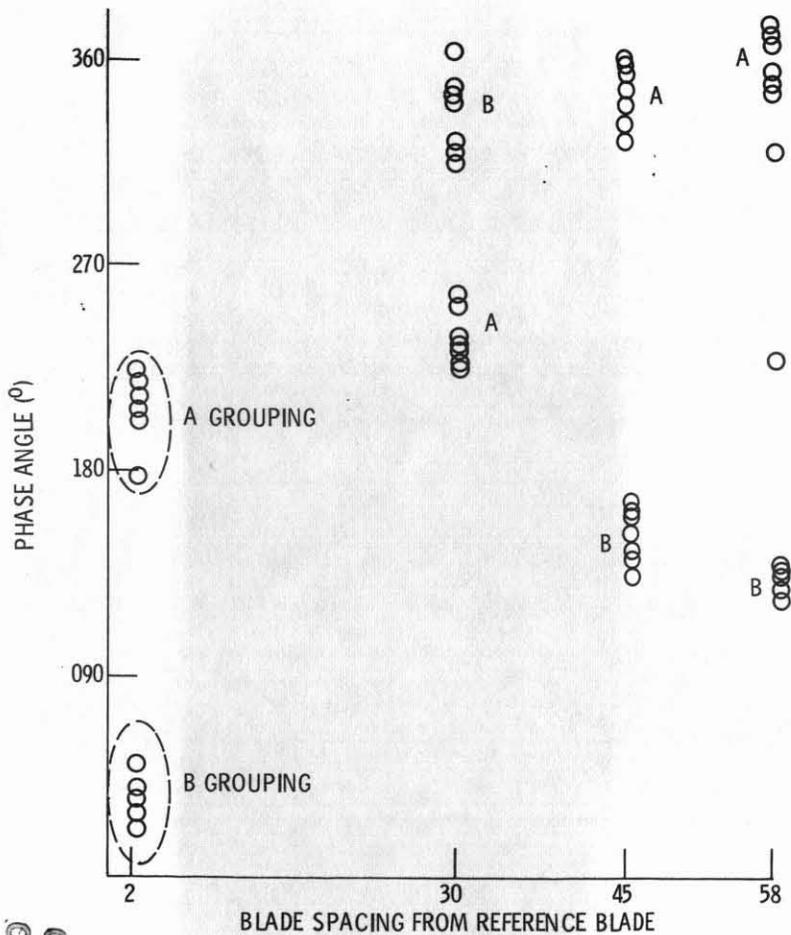
Figure 17. - Phase angle distribution for choke flutter.
