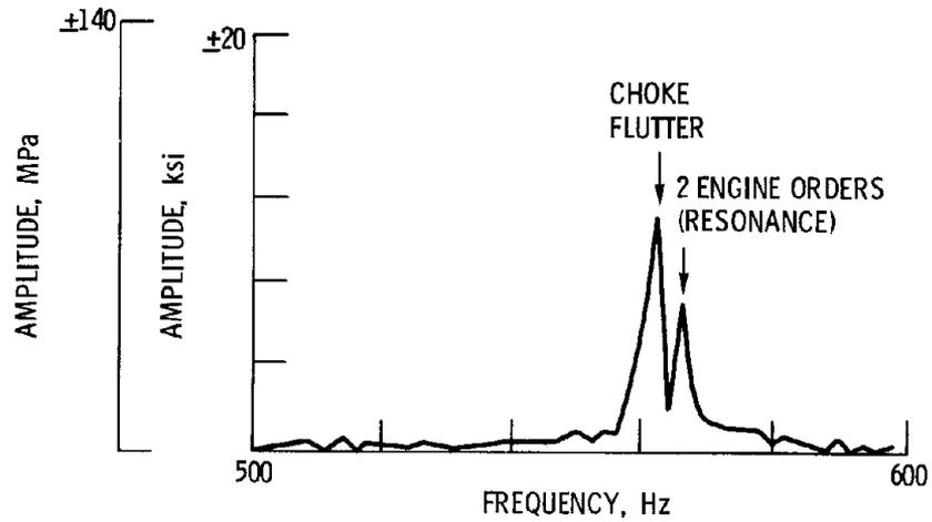
Figure 15. - Choke flutter strain gage spectrum.
