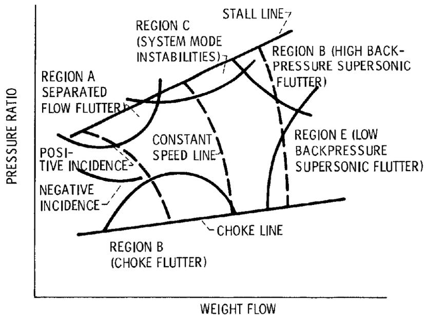
Figure 2. - Compressor performance and revised stability map.
