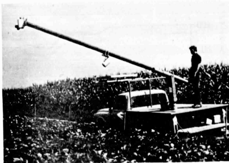
Figure F-1. Truck-mounted multiband radiometer viewing a soybean canopy.
