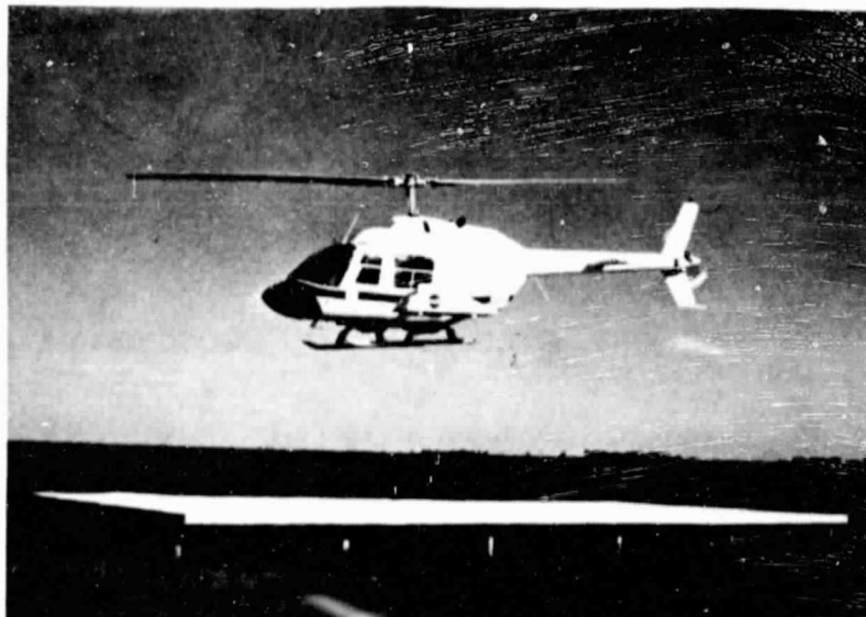
Figure F-12. NASA/JSC field spectrometer system (FSS) viewing canvas reference panel.
