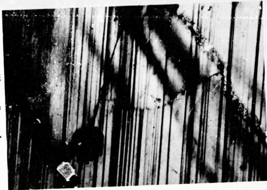
Plate 5. Microfaults in plagioclase megacryst observed under petrographic microscope using crossed nicols. Magnification 20X.
