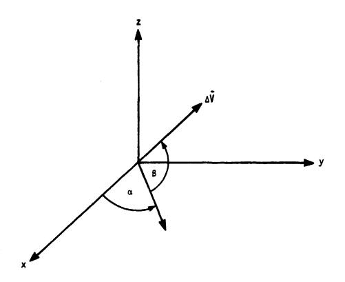
$\Delta \vec{V} = (\Delta \dot{X}, \Delta \dot{Y}, \Delta \dot{Z})$   $\Delta \dot{X} = \Delta V \text{ Cos } \beta \text{ Cos } \alpha$   $\Delta \dot{Y} = \Delta V \text{ Cos } \beta \text{ Sin } \alpha$   $\Delta \dot{Z} = \Delta V \text{ Sin } \beta$
