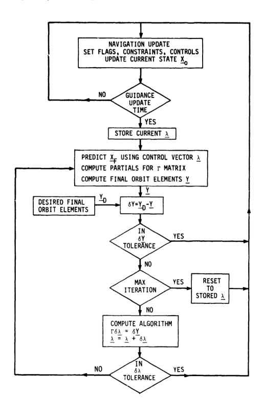
Figure 1-3. GAMMA GUIDE SIMPLIFIED FLOW
