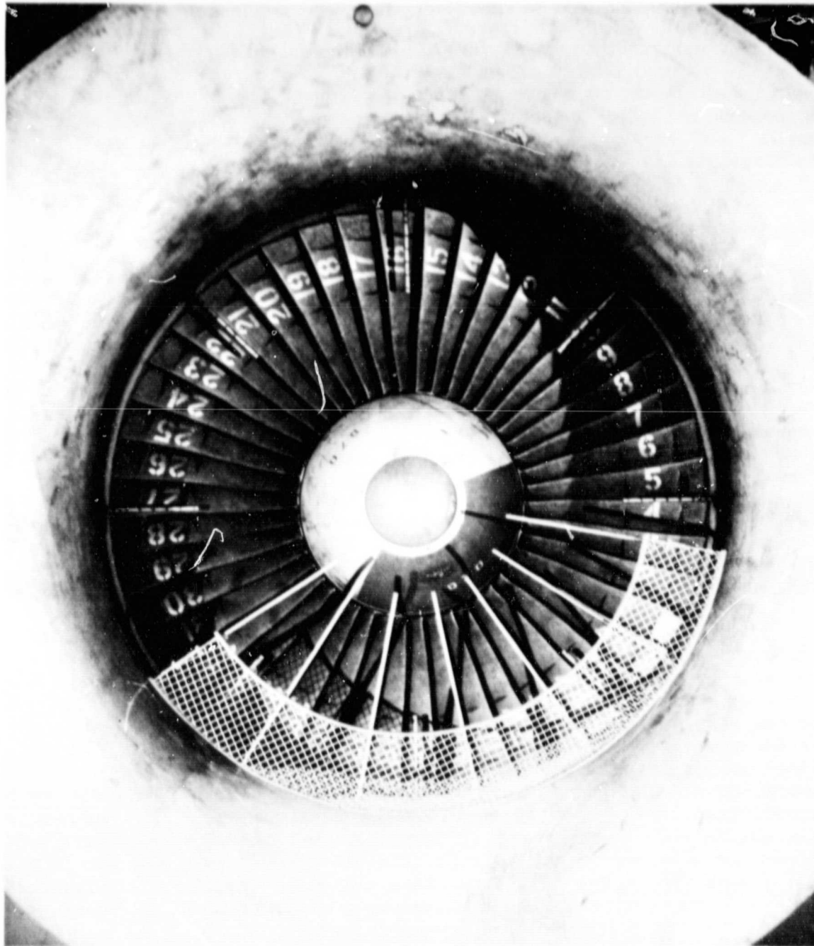
Figure 4-13 Inlet Distortion Screens. Flow blockage induced by these screens simulates the flow distortion that a wing mounted engine would experience at extreme angles of attack.
