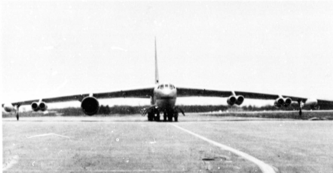
Figure 4-3 B-52 Flying Test Bed. Airplane modifications allow the mounting of an experimental JT9D engine on the right in-board pylon for flight testing.
