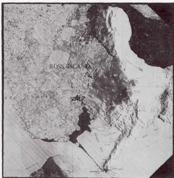
Fig. 7: Part of scene 1174-19433, covering Ross Island, Antarctica, - from Fig. 6 - has been overlaid by cartographic line work to support New Zealand's Antarctic mapping programme.
