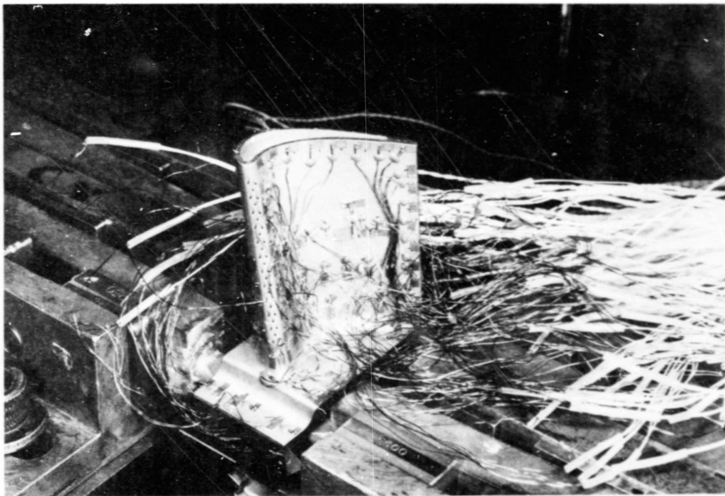
Figure 39. Closeup View of Strain Distribution Test Setup (Stage 1 Blade Shown).
