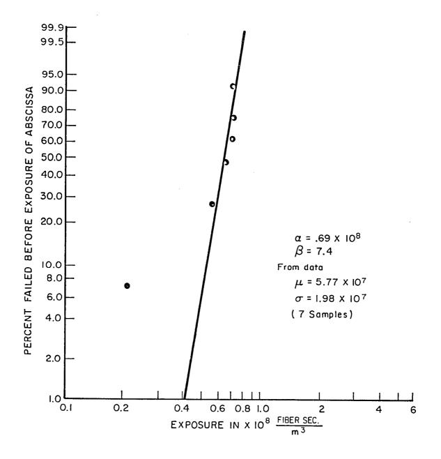
FIGURE 3.1 EXPOSURE TO FLASHOVER FOR WET 7.5 kV PIN INSULATOR, 2mm FIBER.
