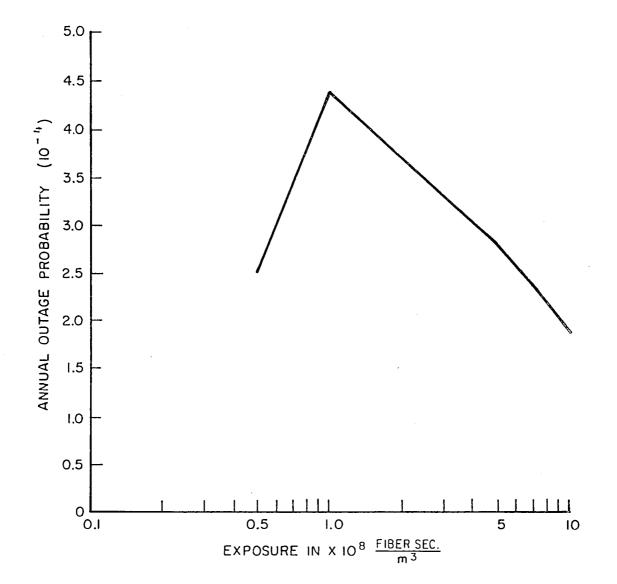
FIGURE 3.5 - ANNUAL OUTAGE PROBABILITY VERSES EXPOSURE LEVEL FOR 15kV POWER SYSTEM plotted as a function of exposure level and displays a clear peak in the vicinity of 1 x  $10^8$  fiber-sec/m<sup>3</sup>.
