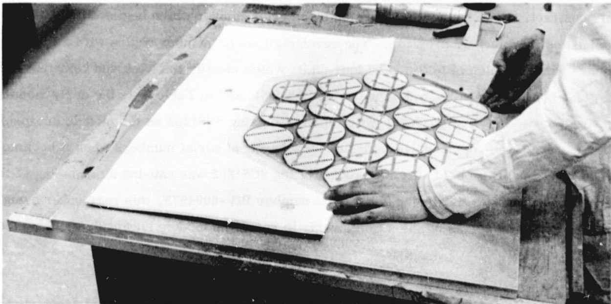
(b) Positioning Coverplate Subassembly
