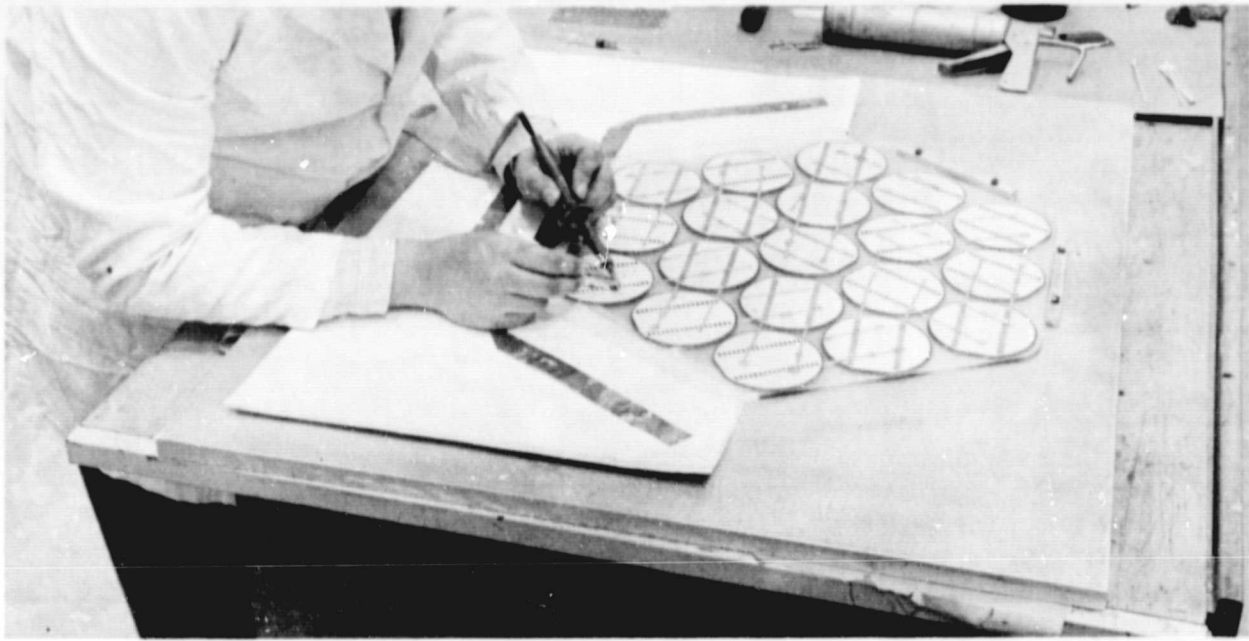
(e) Soldering Positive Termination Strip
