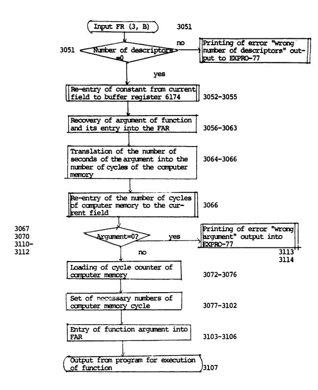
Figure 3. Algorithm of Program that Realizes a Delay in the Fulfillment of the Program
