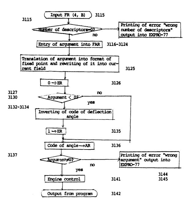
Figure 5. Algorithm of Program Interface for Realization of Function to Control Engine
