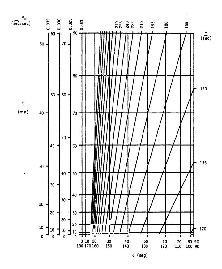
The standard deviation of the single axis IMU alignment error is plotted as a function of the spatial and temporal star pair separations in Figure 4.2-1. The empirically derived value for  $\sigma_0$  was used to generate the plot. There are several time scales corresponding to different values of the standard deviation in the single-axis IMU drift rate.
