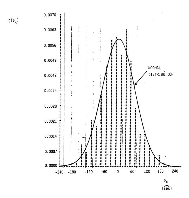
FIGURE C-3 Y-AXIS IMU ALIGNMENT ERROR PROBABILITY DENSITY FUNCTION
