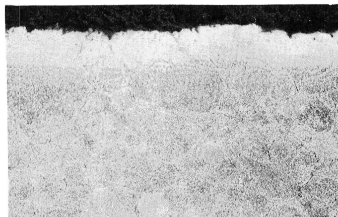
Figure 4-8. Udimet 1008 Can Material - 1st Subscale Run Forged Preforms Surface Reactions (Walker's Etch, 250X)
