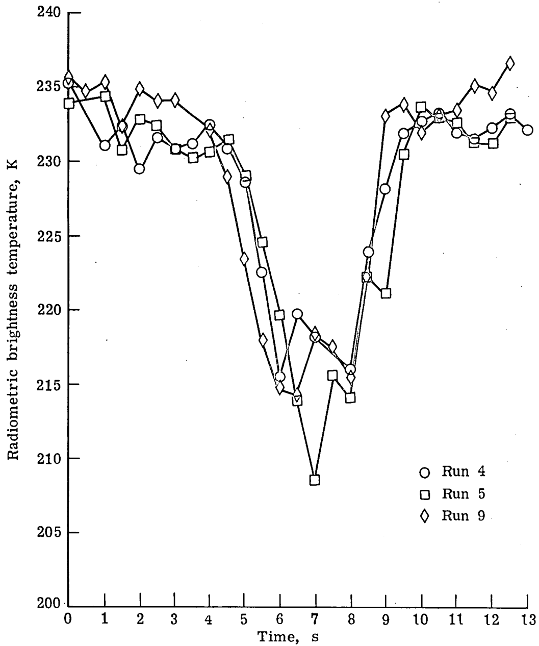
Figure 5-16. Radiometric brightness temperature of the frequency sensitive sea ice versus time for runs 4, 5, and 9 at a frequency of 5.6 GHz.
