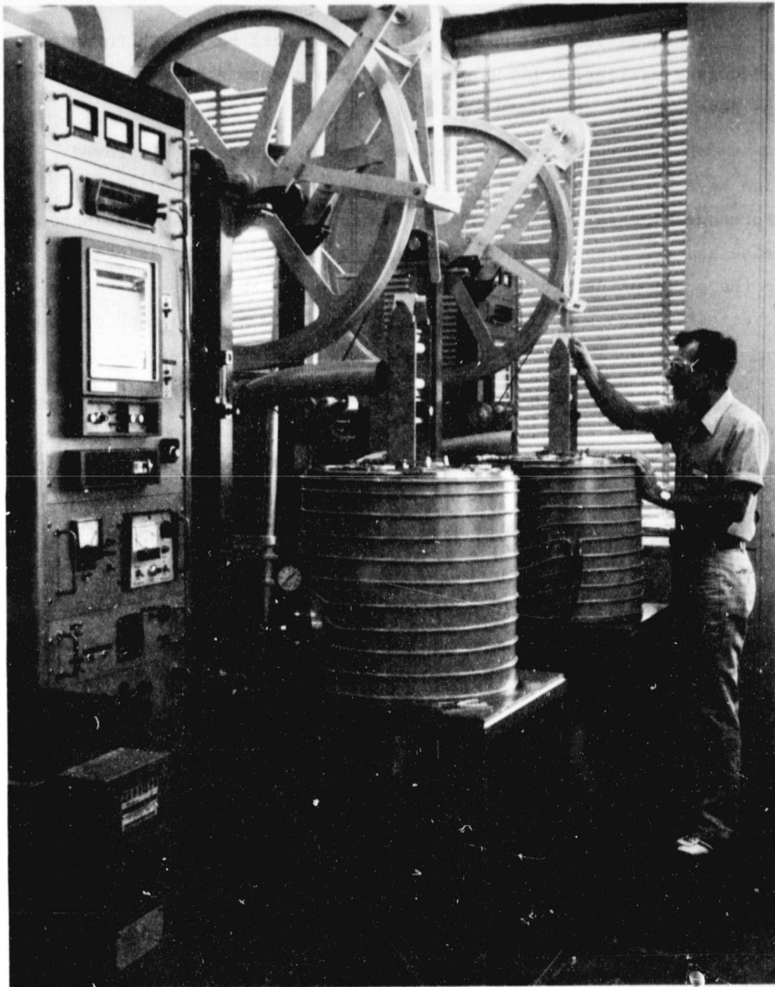
Figure 27 Improved Design Web Furnaces
