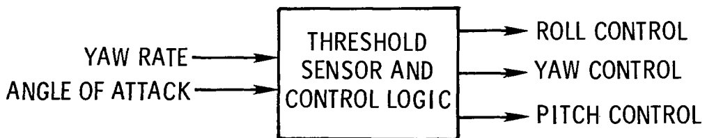
Figure 24. - Conceptual illustration of implementation of automatic spin-prevention systems.
