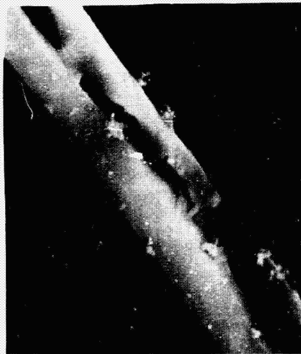
Figure 12.- Scanning electron photomicrograph of irregularly burned carbon fiber.
