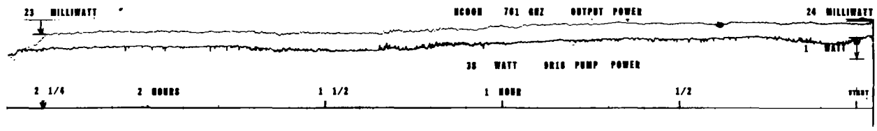
Figure 6.- Long term power stability. Upper trace: 761 GHz line of HCOOH, lower trace 9R18 pump power. Both baselines are heavily offset.
