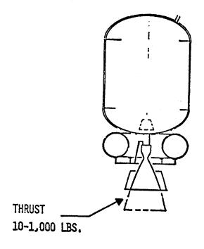
This chart shows that the new chemical program that we are talking about is in the ten to thousand lb. thrust range and a specific impulse which is close to 500 sec. The state-of-the-art drops off very rapidly in the low thrust range. This is why we are speaking of a dedicated thrust system in the low thrust range. There are other programs in the thousand lbs. and higher thrust range that are used for orbital transfer. I am not discussing that today.
