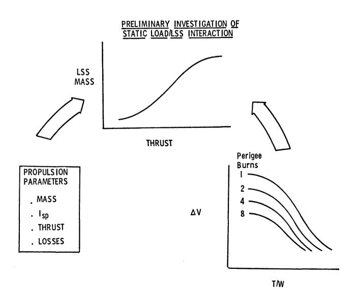
By combining information from figures 14 and 15, LSS area as a function of thrust level may be obtained. We are interested in obtaining a spectrum of such data in order to span the region of interest and understand the relationship between propulsion system thrust level and LSS area.
