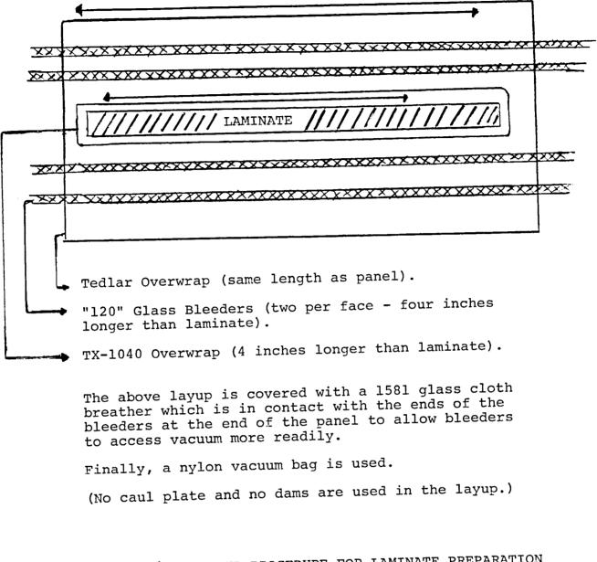
FIGURE 4. LAYUP PROCEDURE FOR LAMINATE PREPARATION (FIRST STAGE)
