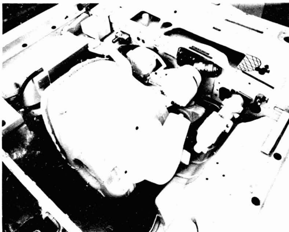
Photographs of Foam Model used to Check Engine Installation In Vehicle
