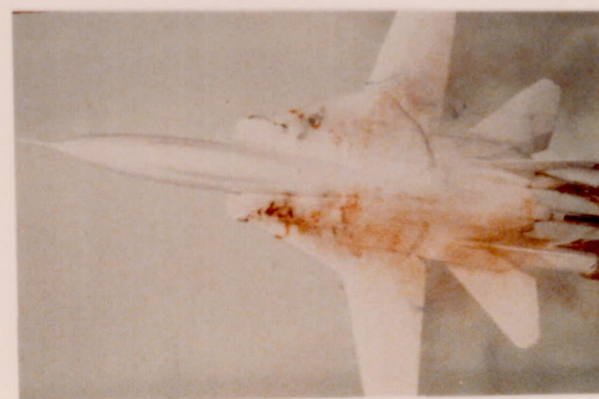
FIGURE 7. EFFECT OF SIDESLIP ON WING-GLOVE FLOW FIELD, \beta = 10^\circ
