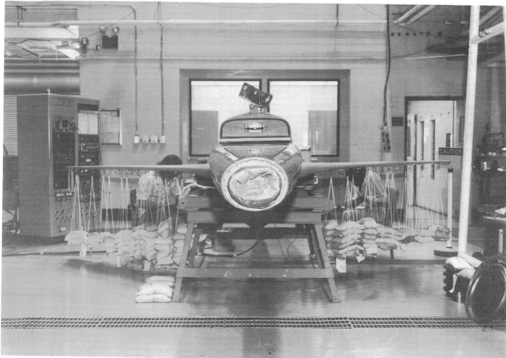
Figure 5.- Photograph of aircraft and wing inverted during loading procedure.
